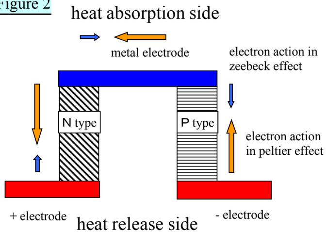
Our dual module consists of Peltier devices. They are combined in a dual layer with thin film sandwiched between metal electrodes drawn in blue in the figure 2. Now, patent is pending. Please contact representative given below for detailed technical inquiry or asking for sample.
